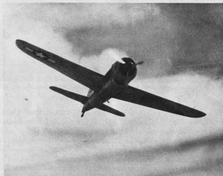
Judy 33, now being produced in great numbers, differs recognitionally from model 11 only by the rounded nose given by radial engine.
